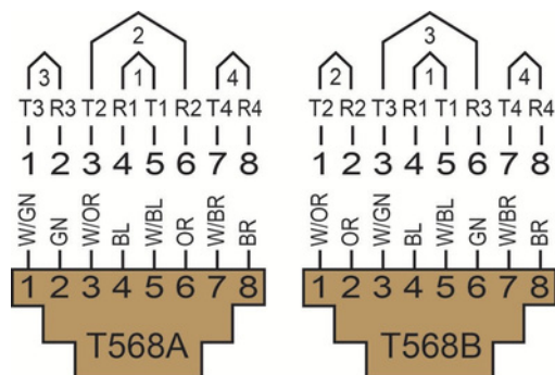
Figure 1: Wiring Schemes
