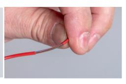
The Jonard Tools BTR-6 Buffer Tube Ring tool provides quick access to fibers inside buffer tubes from 1.2 mm to 6 mm in diameter and will work with buffer tubes with wall thicknesses from 0.2 mm to 0.5 mm. The tool is light and durable with a hardened steel blade for long life and includes a hole for tethering. Easy to use:
