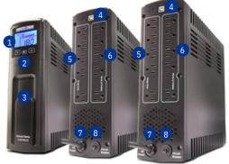
1 LCD Status Display 2 On/Off/Test, Display Scroll, Alarm Silence 3 Tool-less battery access panel 4 USB Communication Port 5 Surge-only 5-15R outlets (4 - 550 & 700, 5 - 1000 & 1500) 6 Battery Backup & Surge 5-15R Outlets (4 - 550 & 700, 5 - 1000 & 1500) 7 6-ft. Power Cord 8 Input Circuit Breaker
