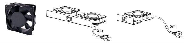
Fan Modules for wall Mounting, ready pre-installed, plug-in and run style , with on/off switches and plugs. Each Fan has an air flow capacity of 2,3-3 cbm/min. Fan Technical data : 18/17 W, 220/240 VAC, 50/60 Hz, 013/0,11 A,2300/3000 rpm 42 - 47 dB noise level
