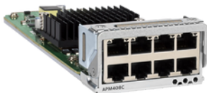
8x10GBASE-T Port Card - 100M/1G/2.5G/5G/10G (APM408C)
