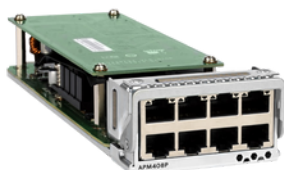
8x10GBASE-T PoE+ Port Card - 100M/1G/2.5G/5G/10G (APM408P)
