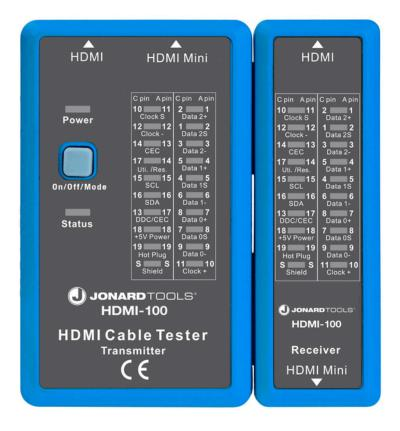
Designed to test HDMI and Mini HDMI cables with ease, this HDMI Cable Tester is the perfect tool for evaluating HDMI cables that may have shorts, open circuits, or have wire pairs in the wrong order. This HDMI tester features the following:
