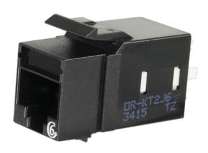
Category 6 Keystone jack, 8-position, 180 degree exit, icon compatible, T568A/B wiring, Black, individually packaged. Keystone, KT2J jacks and modules feature New installer friendly lacing cap termination with free termination tool in every carton. The keystone footprint allows flexibility in installation scheduling because its rear insertion into the faceplate allows the technician to complete the termination before and during the construction process.
