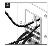
Partially installed openings shall be compressed if left unattended. Excess lubricant is a sign of good compression.
