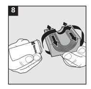
Lubricate the sealing surfaces with Roxtec Lubricant.
