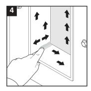
Lubricate the sealing surfaces of the frame. Lubricate the corners thoroughly.
