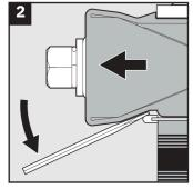
Remove the wedge by lifting it over the stayplate using a flat
