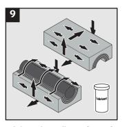
Lubricate the sealing surfaces of any spare module. Do not remove the core.
