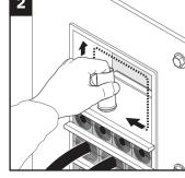
Lubricate the exposed sealing surfaces.
