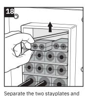
insert the final row of modules between the stayplates.
