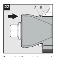
Ensure that the wedge is secured within the stayplate edges. The stop edge (A) is flush to the frame (B).
