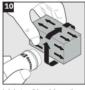
Lubricate solid modules on the sealing surfaces.
