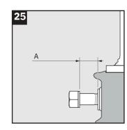
The screwhead will move outwards during tightening. The distance (A) shall accommodate the wedge clip.
