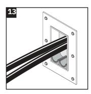
Cables/pipes shall go in parallel with the frame.
