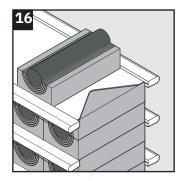
Ensure that the odules are secured within the stayplate edges.
