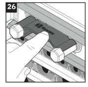
Attach the wedge clip. The wedge clip verifies correctly tightened wedge.
