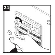
Tighten the screws alternately in small steps until full mechani- cal stop (~25-30 Nm). Protruding excess lubricant indicates a tight
