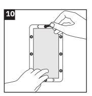
Attach the short sides of the frame to the structure using two of the self-tapping screws.
