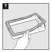
Apply the adhesive gasket onto the frame side that will face the structure. Do not apply it on the side with the hexagonal holes.
