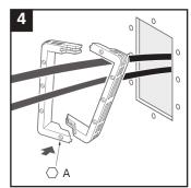
Reconnect the frame parts. Hexagonal bolt holes must point outwards, away from the structure.
