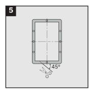
If cables are pre-routed, cut the gasket in a 45° angle.
