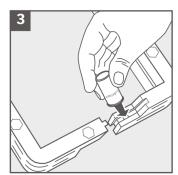
Lubricate all end surfaces of the frame parts with any Roxtec Lubricant.
