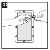
Insert and tighten the rest of the self-tapping screws cross-wise in small steps to 7 Nm. Do this carefully with thin structures.
