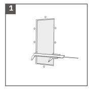
Make or verify an aperture. Maximum structure thickness 4 mm
