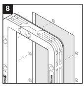
The hexagonal holes shall face outwards.
