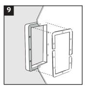
For thin structures of 1.5 millimeters or less a C KFO counterframe shall be used.
